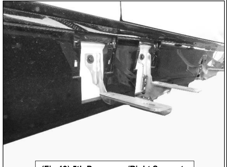
(Fig 19) 5th Passenger/Right Support Bracket attached.
