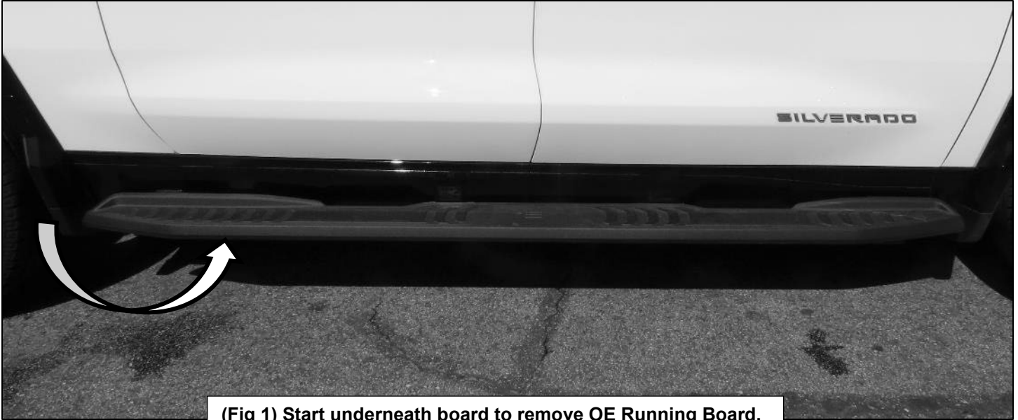
(Fig 1) Start underneath board to remove OE Running Board.
